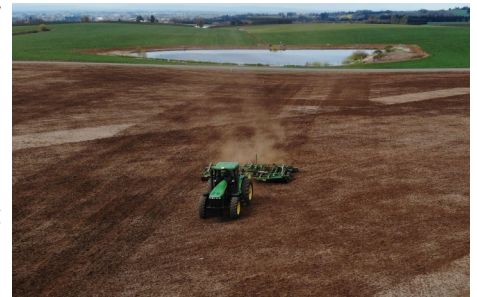
Great Plains Turbo Max minimum tillage tool preparing a field for fine fescue planting.
